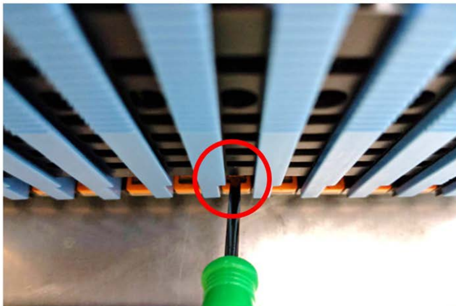
Figure 2.2 Unlock the latch to remove the module
