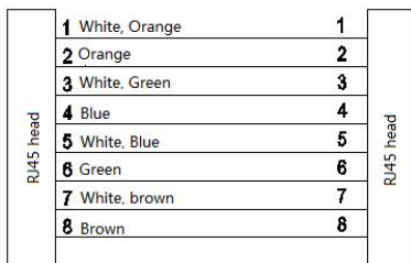
Figure 3-2 Five-category straight-through network cable wiring method
