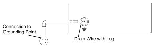
**Figure 2.13 Grounding Connection**
