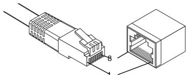
Figure 2.11 Ethernet Plug & Connector Pin Position
