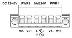
Figure 2.14 Terminal Receptor: Relay Contact
