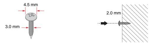
Figure 2.4 Securing Wall Mounting Screws
