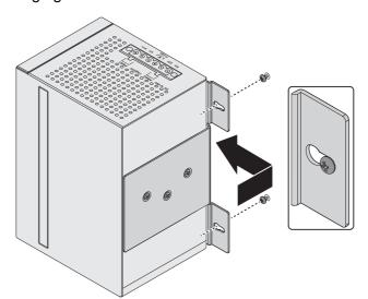
**Figure 2.5 Wall Mount Installation**
