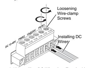
Figure 2.17 Installing DC Wires in a Terminal Block
