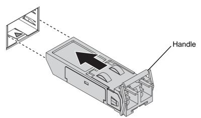
Figure 2.7 Installing an SFP Transceiver
