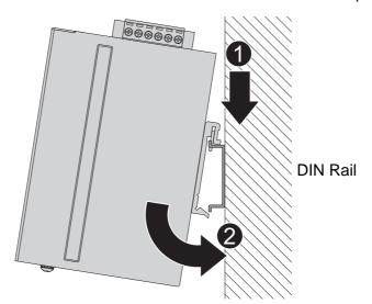
Figure 2.1 Installing the DIN-Rail Mounting Kit
