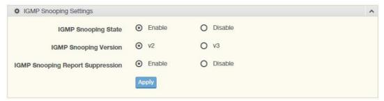
Figure 3.29 L2 Switching > Multicast > IGMP Snooping > IGMP Settings
