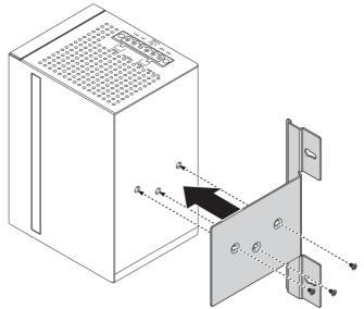
Figure 2.3 Installing Wall Mount Plates
