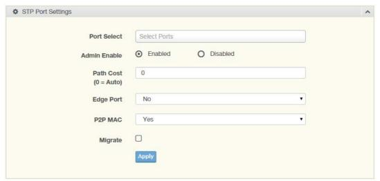
Figure 3.37 L2 Switching > Spanning Tree > STP Port Settings
