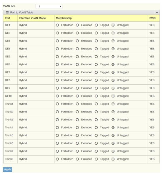
Figure 3.24 L2 Switching > 802.1Q VLAN > Port to VLAN
