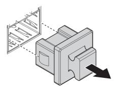
Figure 2.6 Removing the Dust Plug from an SFP Slot
