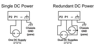
Figure 2.12 Power Wiring for EKI-5500/5600-EI/MB series
