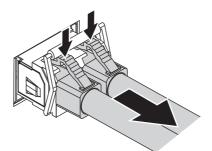
Figure 2.9 Removing a Fiber Optic Cable to a Transceiver
