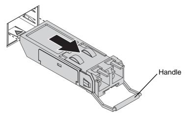
Figure 2.10 Removing an SFP Transceiver
