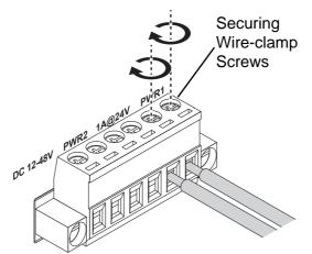
Figure 2.18 Installing DC Wires in a Terminal Block
