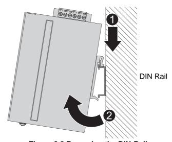
Figure 2.2 Removing the DIN-Rail
