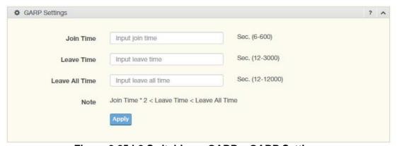
Figure 3.25 L2 Switching > GARP > GARP Settings
