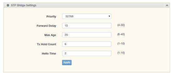
Figure 3.38 L2 Switching > Spanning Tree > STP Bridge Settings
