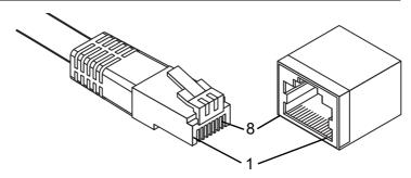
Figure 2.8 Ethernet Plug & Connector Pin Position
