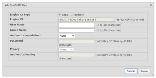
Figure 4.59 System > Advanced Configuration > SNMP > User Security Model > Add
