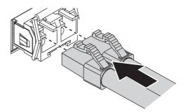
Figure 2.5 Attaching a Fiber Optic Cable to a Transceiver
