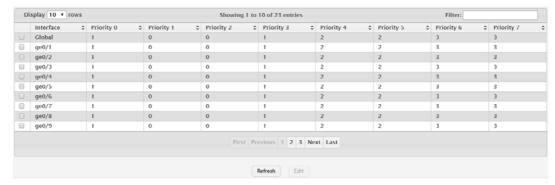
Figure 4.151 Switching > Class of Service > 802.1p
