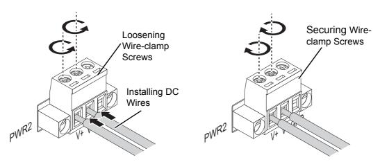
Figure 2.15 Installing DC Wires in a Terminal Block
