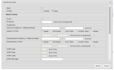
Figure 4.308 QoS > Access Control Lists > Configuration > Add Rule
