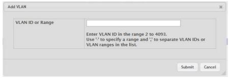
Figure 4.265 Switching > Private VLAN > Configuration > Add VLAN
