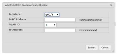
Figure 4.171 Switching > IPv6 DHCP Snooping > Base > Static Bindings > Add The following table describes the items in the previous figure.
