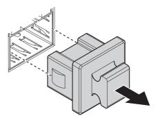
Figure 2.3 Removing the Dust Plug from an SFP Slot
