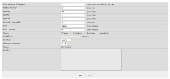
Figure 4.147 System > Utilities > TraceRoute
