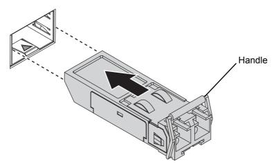
Figure 2.4 Installing an SFP Transceiver
