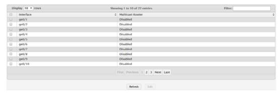
Figure 4.206 Switching > MLD Snooping > Multicast Router Configuration
