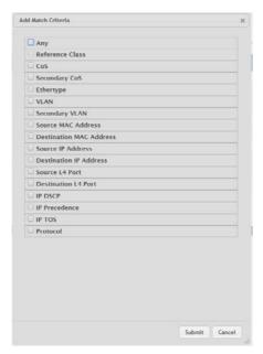
Figure 4.321 QoS > Diffserv > Class Configuration > Add Match Criteria
