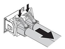
Figure 2.7 Removing an SFP Transceiver
