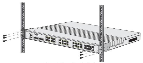
Figure 2.2 Installing the Switch
