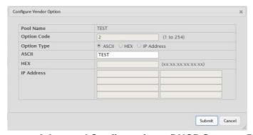
Figure 4.18 System > Advanced Configuration > DHCP Server > Pool Options > Configure Vendor Option
