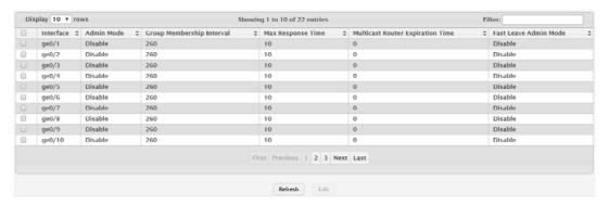
Figure 4.191 Switching > IGMP Snooping > Interface Configuration
