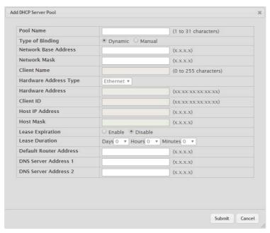
Figure 4.14 System > Advanced Configuration > DHCP Server > Pool Summary > Add
