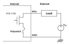
Note \*: When a inductance load is connected, the maximum output voltage will be 24 V.
