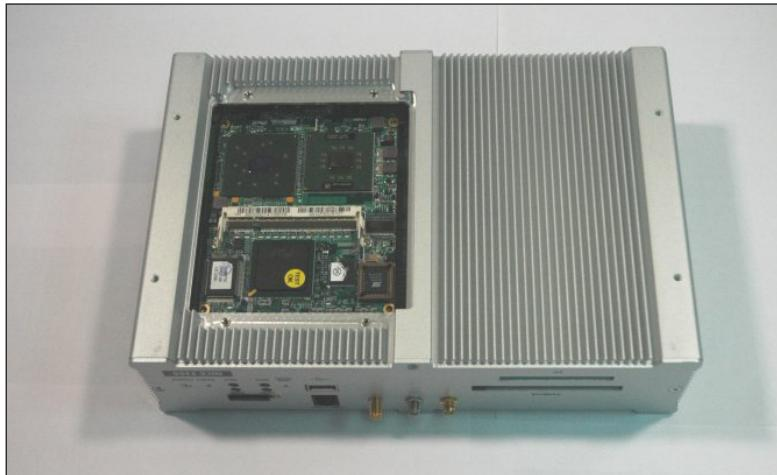
2. When all the connectors are aligned, firmly but gently press down the four corners of the ICES 101 module until the connectors are firmly seated in the slots.
