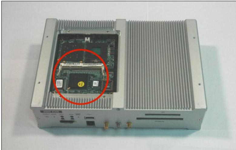
2. Insert the SODIMM into the slot at a 45-degree angle, and then push it in until the gold-plated connector is seated firmly in the slot.
