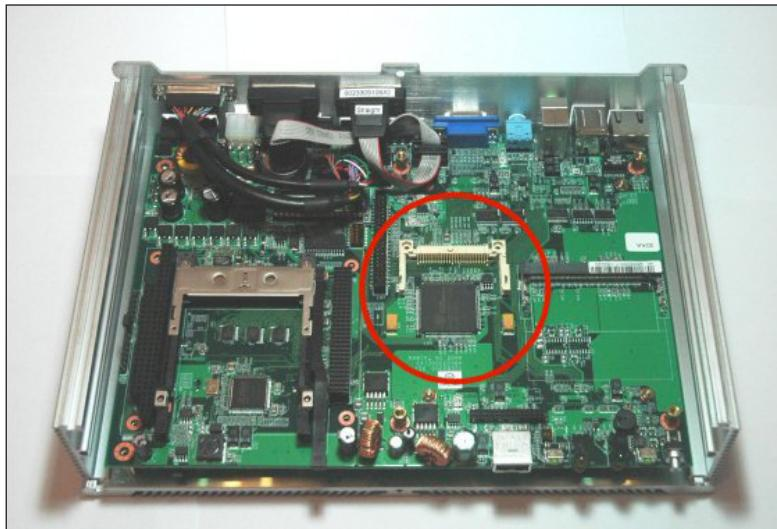
2. Insert the CF card into the socket with the label facing up.
