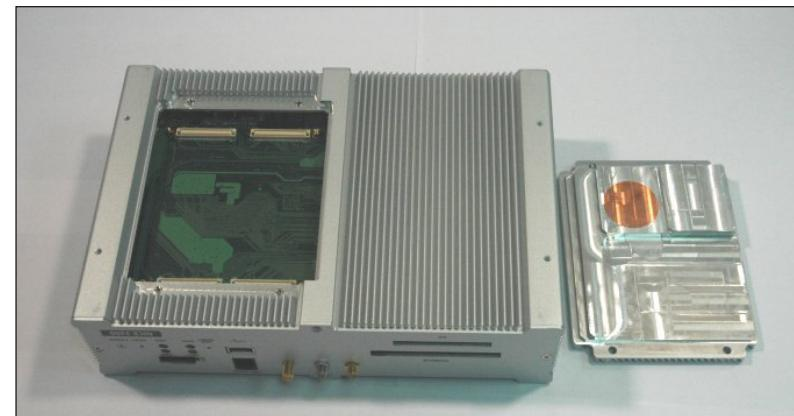
You are now ready to install the ICES 101 module and SODIMM. Note that there are two types of heatsink for the ICES 101 module – an onboard CPU type (C65 and 373) and a socket CPU type (SKT). Make sure you use the correct heatsink for the ICES 101 module that you are installing.
