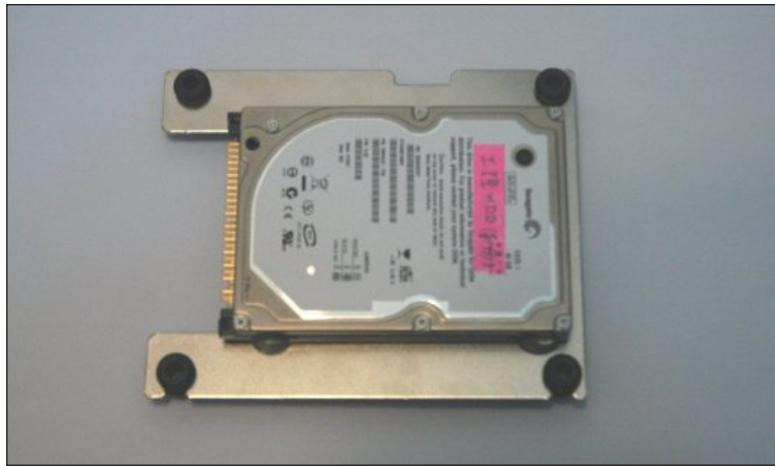
8. Replace the mounting bracket on to the board, ensuring that the screw holes on the bracket are aligned with the screw holes on the board.
