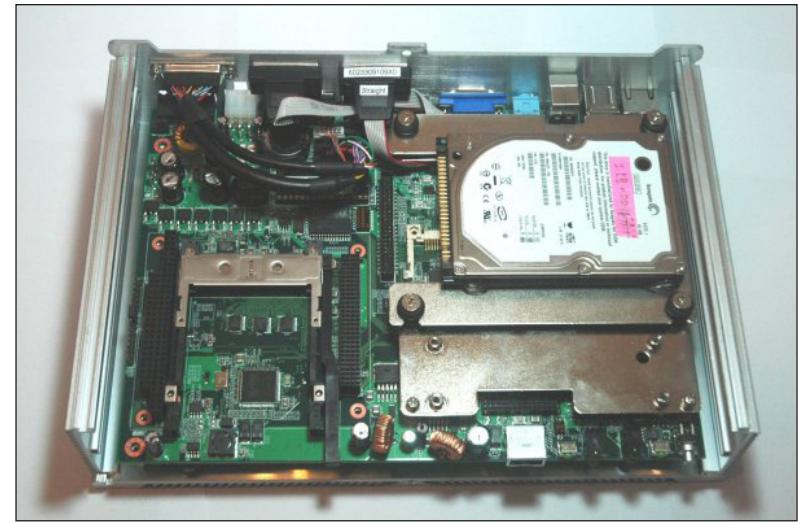
9. Secure the mounting bracket to the board using the four screws that you removed in Step 2.
