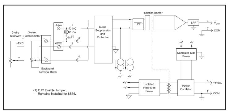
Figure 1: 8B36 Block Diagram
