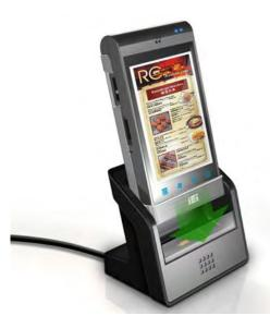
Figure 2-6: Connect the MODAT-200 to the Charging Cradle
