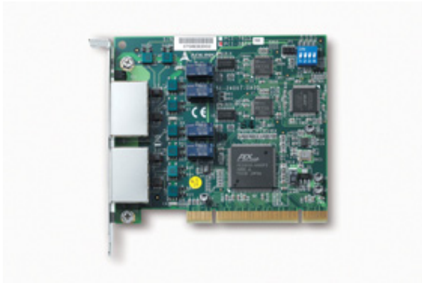
Figure 2-1: PCI-7854 front view
