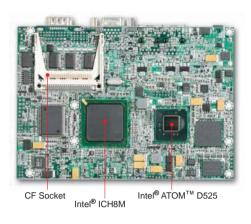
PEB-2771/2781 take advange of the latest Intel® Atom™ technologies. It support DDR3 SDRAM, dual gigabit ethernet and one expansion Mini PCI Express x1 socket. Base on leading Intel<sup>®</sup> Atom<sup>™</sup> solution , PEB-2770/2780 performs low power dissipation, high performance and fanless requirement. Therefore, it's applied to Panel PC, Kiosk, DS, Medical, Military and industrial automation.
