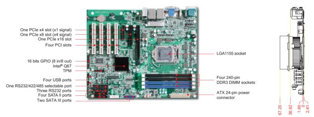
With the Intel® Q67 chipset on board, the RUBY-D712VG2AR supports the latest quad-core 2nd Generation Intel® Core™ i7 and Core™ i5 processors. This model is also ideal for Factory Automation, Medical, Gaming, Digital Signage, Surveillance Security Monitoring and Kiosk with high performance requiring various I/O connectors.
