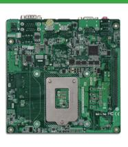
WADE-8210-H110 is based on Intel® H110 chipset and Desktop processors including Intel®  $7^{th}$  and  $6^{th}$  Gen Core<sup>TM</sup> i3/i5/i7 SKU. This board supports DDR4, PCIe 3.0, and SATA III. Those features help you to build high performance and stable system.
