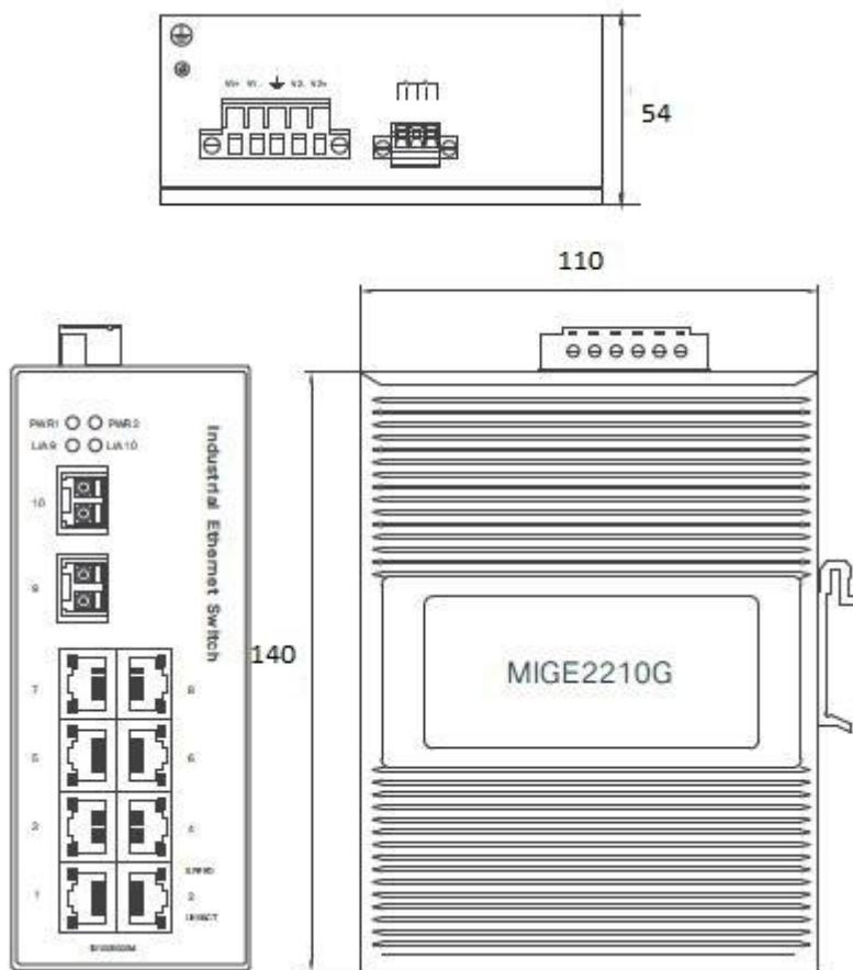
Din-rail mounting (unit: mm)
