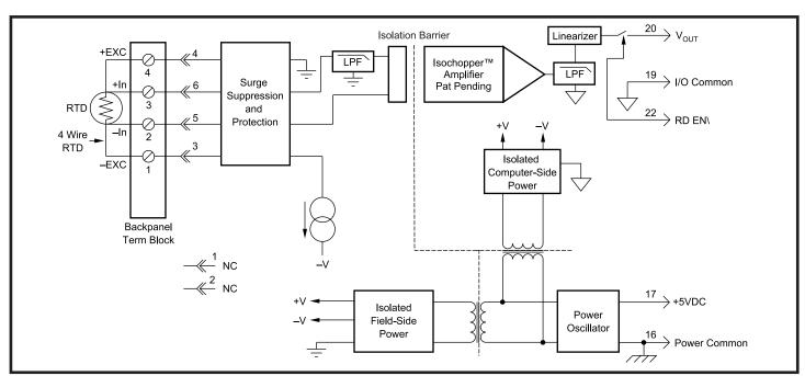
Figure 1: SCM5B35 Block Diagram
