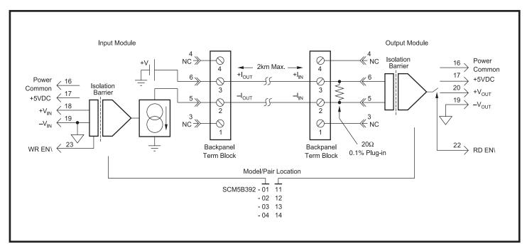
Figure 1: SCM5B392 Block Diagram
