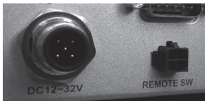
M12 type power connector and remote switch connector
