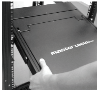
2. Slide the LCD KVM Switch onto the rails and secure it to the rack.
