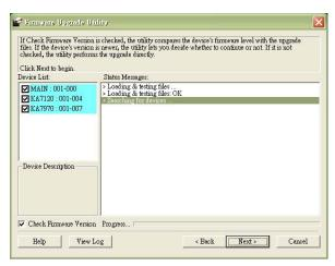
The Utility checks to make sure the KH1508A / KH1516A is in the Firmware Upgrade Mode and then lists all firmware needed preselected in the *Device List* panel.
