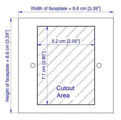
**Note:** ATEN recommends a 1-gang wall box with a depth of at least 4.5 cm (1.77 inches) to accommodate the connectors and cables.
