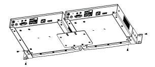
5. Screw the mounting brackets onto the rack.
