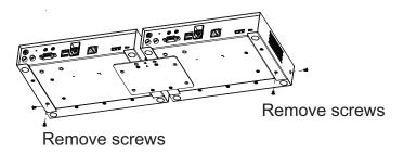
3. Use the screws in step 2 to install the left and right mounting brackets.
