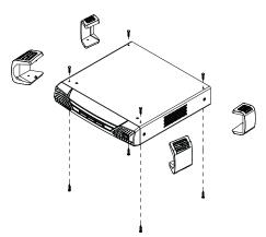
2. Remove the bottom and side screws from the unit.
