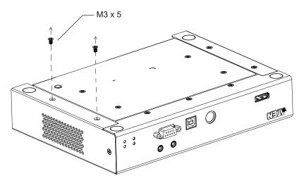
2. Use the screws from step 1 to attach the mounting bracket to the bottom of the transmitter, as shown below.
