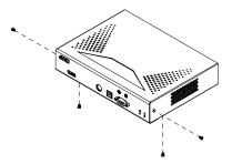
3. Use the screws in step 2 to install the right and left mounting brackets.
