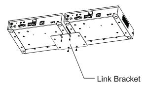
2. Remove the bottom and side screws from each unit.
