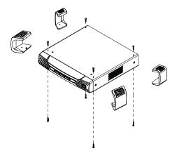
2. Remove four screws from the units and then use the same screws to secure the units together with the link bracket provided with the kit.
