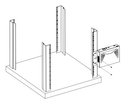
Note: Rack screws are not provided. We recommend the use of M5 x 12 Phillips Type I cross recessed screws.
