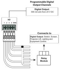
Digital outputs provide non-powered dry contact (open and closed) circuit control of devices, which must be connected using a **relay module**.
