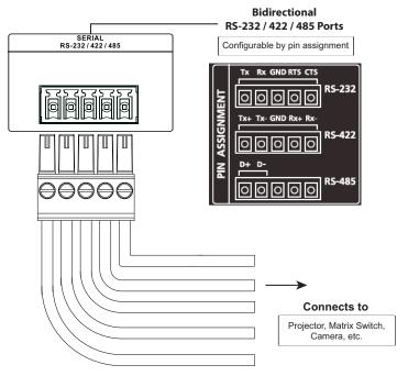
Connect to devices, configurable by pin assignments, for controlling and receiving status messages from them.
