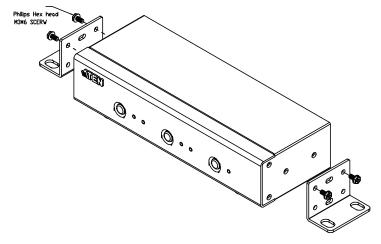
2. Screw the bracket into a convenient location on the rack.
