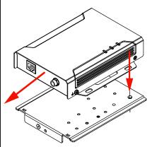
Step A: Put on plate, fit mounting post, and slide forward.
