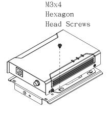
Step B: Screw device to mounting plate.
