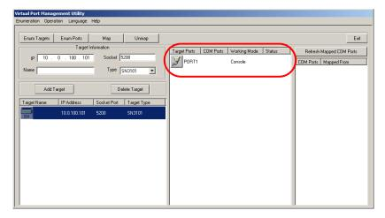
• The left column lists the target's port number, the second column shows the COM port it is mapped to (if any), the third column shows its working mode, and the right column shows its status.
