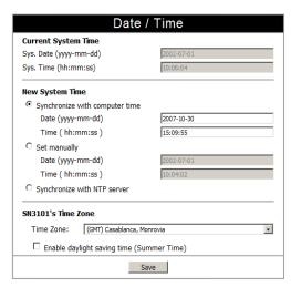
The date and time that the SN3101 is currently set to appear in the upper section. The large lower section offers three methods to set new date and time parameters:
