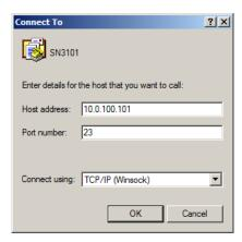
3. For the *Connect using:* field, select TCP/IP (Winsock); then click OK. HyperTerminal opens up a Telnet session and you can log in to the SN3101 with your Username and Password to bring up the SN3101's Main Menu. See *Telnet*, page 31 for Telnet operation.
