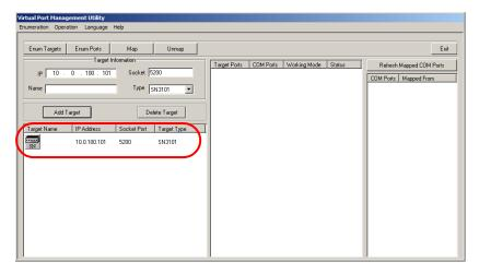
**Note:** Double clicking an item in the list invokes the same function as selecting **Enum Ports** – which displays the numbers and working modes of the selected target's ports in the *Port List* column.
