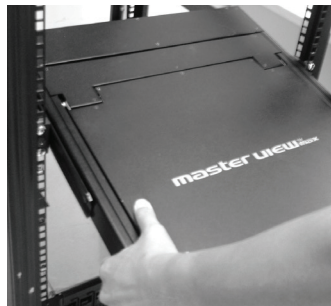
2. Slide the LCD KVM Switch onto the rails and secure it to the rack.
