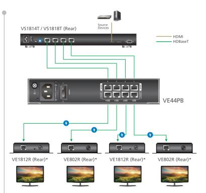
\*Power can be supplied to the POH-powered device through HDBaseT transmission (no need for a power adapter).
