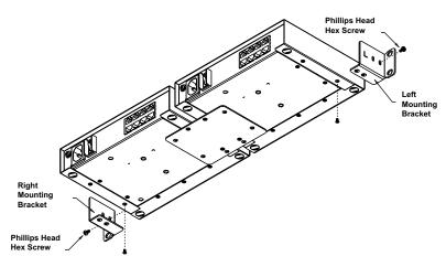
4. Screw the mounting brackets to the rack.
