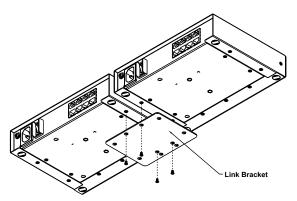
2. Remove the bottom and side screws from each VE44PB unit.
