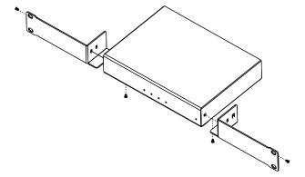
3. Screw the mounting brackets to the rack.
