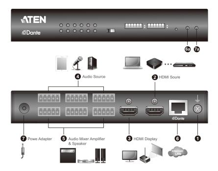
Ground the VE66DTH by connecting one end of a grounding wire to the ground terminal and the other end to a suitable grounded object.
