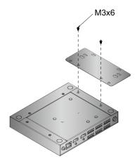
2. Screw the bracket into any convenient location on the rack.
