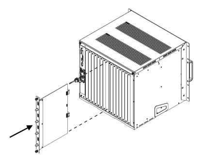
3. Slide an input board into a right side slot and then tighten the screws to secure the board to the VM3200 / VM3250.
