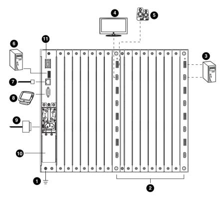
1. Use a grounding wire to ground the unit by connecting one end of the wire to the grounding terminal, and the other end of the wire to a suitable grounded object.
