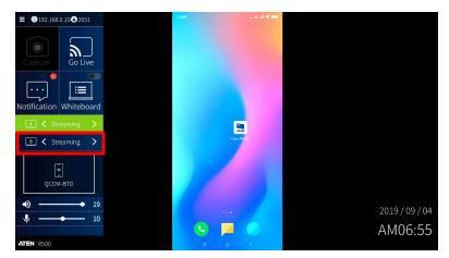
Use the left and right Navigation pushbuttons/buttons to select the source. In this example, Display B is switched from streamed-in sources to HDMI. 4. Now you have successfully switched the display source from streaming to HDMI for display B.
