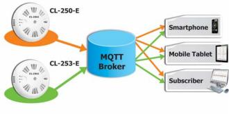
Supports the MQTT Protocol for IoT Applications
