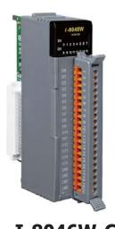
**I-8046W-G**16-channel Isolated Digital Input Module
