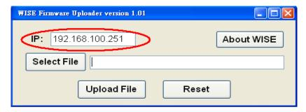
Figure 10-10: Assign IP address
