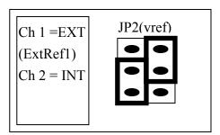
If JP2 select **internal reference**, then JP1 select **-5 V/-10 V** internal reference voltage. If JP2 select **external reference**, then **ExtRef1**, **CN3 pin 31**, is the external reference voltage for DA channel 1; and **ExtRef2**, **CN3 pin 12**, is the external reference voltage for DA Channel 2. If user provides AC +/- 10 V external reference voltage, the D/A output voltage may be AC -/+ 10 V
