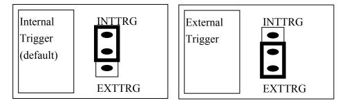
The A-823PGL/PGH supports two trigger type, **internal trigger** and **external trigger**. The external trigger comes from **ExtTrg**, **CN3** pin 17. There are two types of internal trigger, **software trigger** and **pacer trigger**. The details information is given in section 2.4.8.
