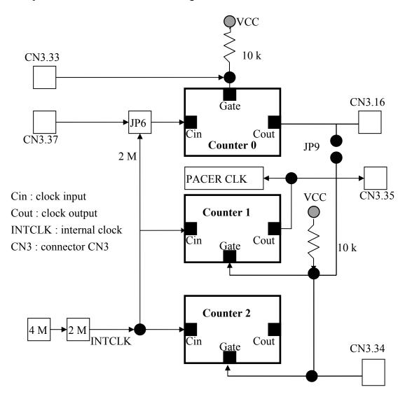
The counter0, counter1 and counter2 are all 16 bits counter. The COUT of counter 0 can control counter 1 gate by JP9 setting. The counter1 is a 16 bits timer is used as <u>pacer timer</u>. The software driver, A823\_Delay(), uses counter 0 to implement a machine independent timer for settling time delay (sec. 2.4.6 and sec. 2.4.7). If user doesn't use A823\_Delay(), the counter0 can be used as a general purpose timer/counter.
