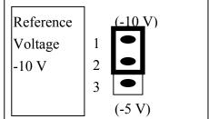
Select (-5 V) : D/A voltage output =  $0 \sim 5$  V (both channel) Select (-10 V) : D/A voltage output =  $0 \sim 10$  V (both channel)
