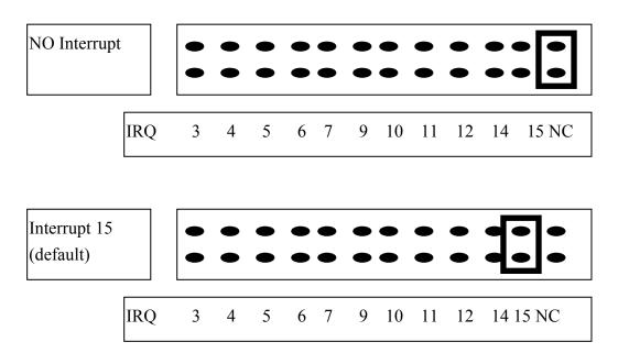
The interrupt channel <u>can not be shared.</u> The A-823 software driver can support 8 different boards in one system but only **2 of these cards** can use interrupt transfer function.
