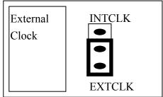
The A-823PGL/PGH has 3 independent 16 bits timer/counter. The cascaded counter1 and counter2 are used as **pacer timer**. The counter0 can be used as a user programmable timer/counter. The user programmable timer/counter can select **2 M internal clock** or **external clock ExtCLK, CN3 pin 37**. The block diagram is given in section 2.6. The clock source must be very **stable.** It is recommended to use internal 2 M clock.
