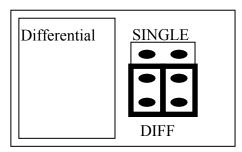
The A-823PGL/PGH offer 16 single-ended or 8 differential analog input signals. The JP3 select single-ended/differential. The user can not select single-ended and differential simultaneously.
