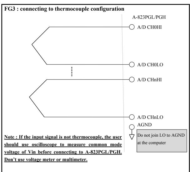
**CAUTION**: In Fig3, the maximum common mode voltage between the analog input source and the AGND is  $70 \ V_{D-D}$ , so the user must make sure that the input signal is under specification first. If the common mode voltage is over  $70 \ V_{D-D}$ , the input multiplexer will be damaged forever.
