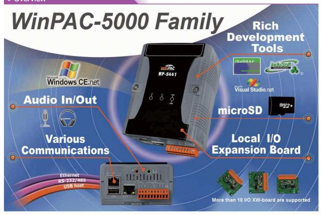
The ICP DAS WinPAC-5000 Series is the new generation PAC (Programmable Automation Controller). It is equipped a PXA270 CPU (520 MHz) running a Windows CE.NET 5.0 operating system, various connectivity (VGA, USB, Ethernet, RS-232/485) and I/O expansion bus.
