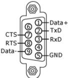
COM3 can be configured as either RS-232 or RS-485 that only can select one at a time; its configuration depends on the pin connections as follows:
