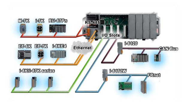
Beside the local I/O slots, iPAC-8000 also equips several RS-232/485 ports, two Ethernet ports to connect serial I/O and Ethernet I/O. And with FRnet and CAN communication module in local slot, FRnet I/O and CAN devices are easy to be integrated.
