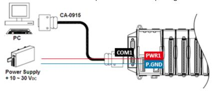
For Ethernet controllers, you also can connect to PC using an Ethernet cable.
