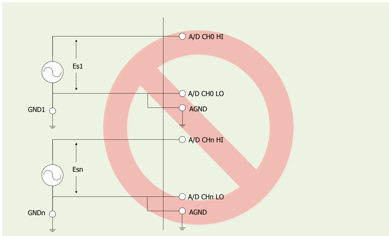
■ Figure2.4-2: Grounded loop input (Wrong way)
