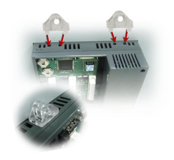
Step 4: Screw the panel mounting clips to the panel
