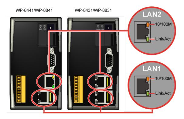
Each Ethernet port has two LED indicators, which are used to indicate the network speed and Link/Acting, as described below.
