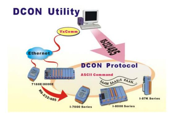
The DCON Utility is a toolkit that help user search the network, easily to Configure the I/O modules and test the I/O status via the serial port (RS-232/485) or Ethernet port (using virtual com port). It supports not only the DCON Protocol I/O modules but also the M Series I/O Modules (Modbus RTU M-7K, M-87K and will support Modbus ASCII M-87K) now.
