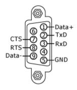
COM3 can be configured as either RS-232 or RS-485, but only one mode can be selected at a time and the configuration depends on the pin connections as described below.
