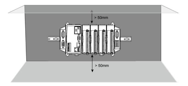
There is a minimum of 50mm clearance between the top and bottom edges of the WinPAC and the enclosure panels.
