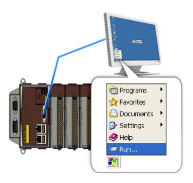
Step 16: On the "Run" dialog, type the command which displays in step 5 and then click the "OK" button
