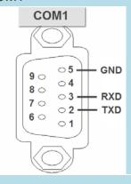
(RS-232 used to update firmware) Note: CPU internal UART
