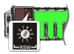
Turn the rotary switch to "3", and then reboot the WinPAC.
