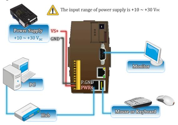
The diagram below shows the connections of 4/8 slots module of the WinPAC.
