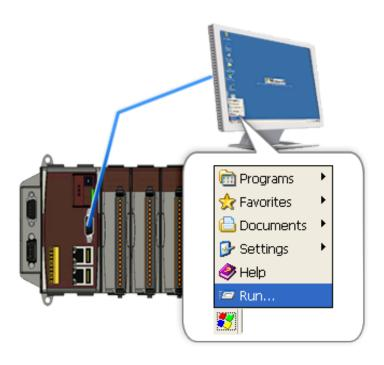
Step 8: On the "Run" dialog, type the command which displays in step 6 and then click the "OK" button
