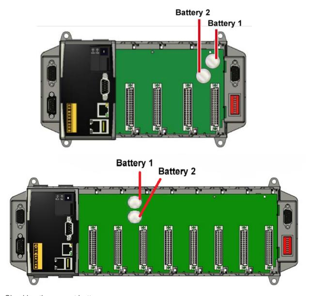
Checking the current battery power:
