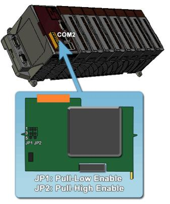
When WinPAC as a master using COM3 communication interface, the pull-high/pull-low resistor located on the power board must adjust to enable as shown below.
