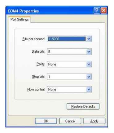
Figure 24 Setting Port Parameters
