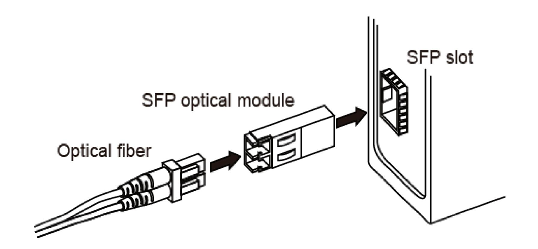
Figure 14 Connecting the SFP Optical Module
