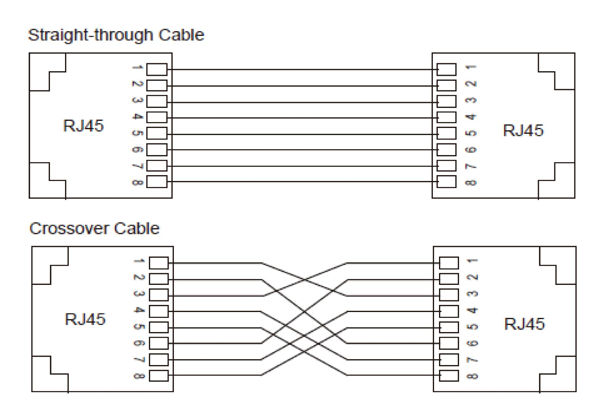
Figure 11 Connection Using Straight-through/Cross-over Cable
