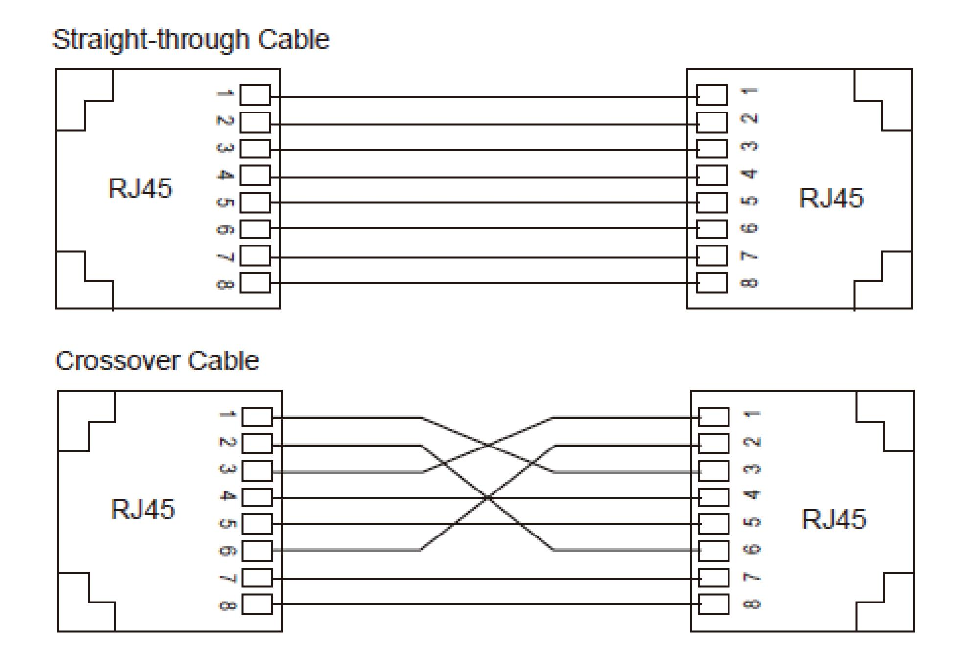
Figure 8 Connection Using Straight-through/Cross-over Cable
