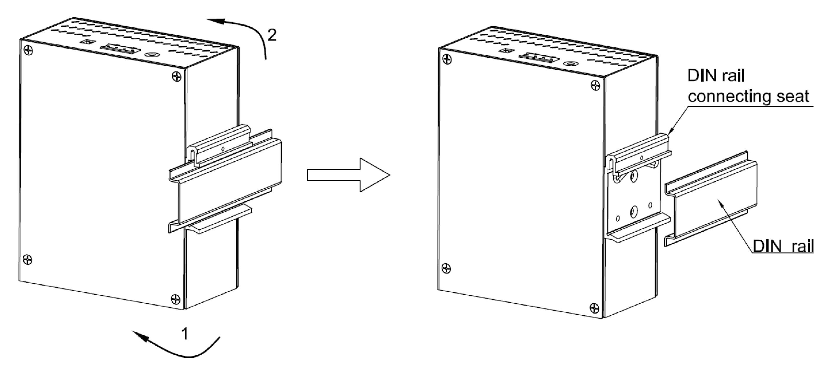
Figure 6 DIN Rail Dismounting
