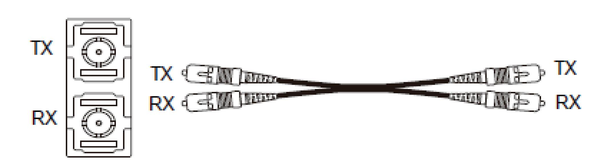
Figure 9 Connection of 100Base-FX Ethernet Port
