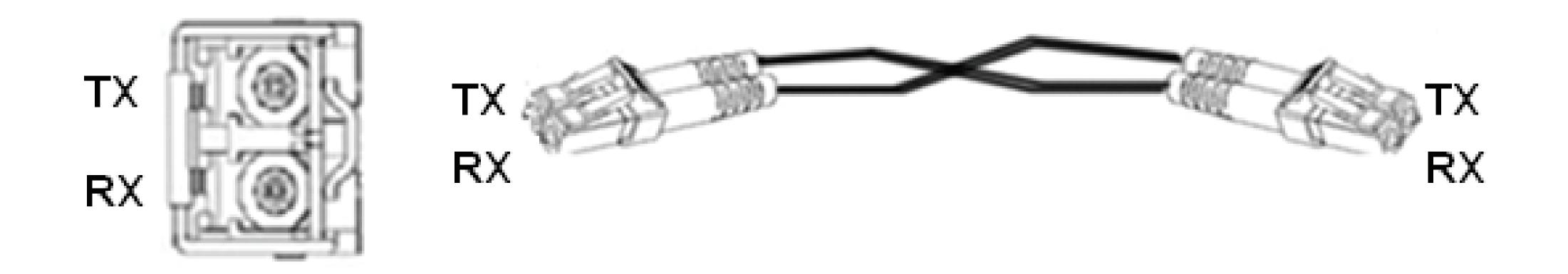
Figure 13 Fiber Connection of an SFP Optical Module
