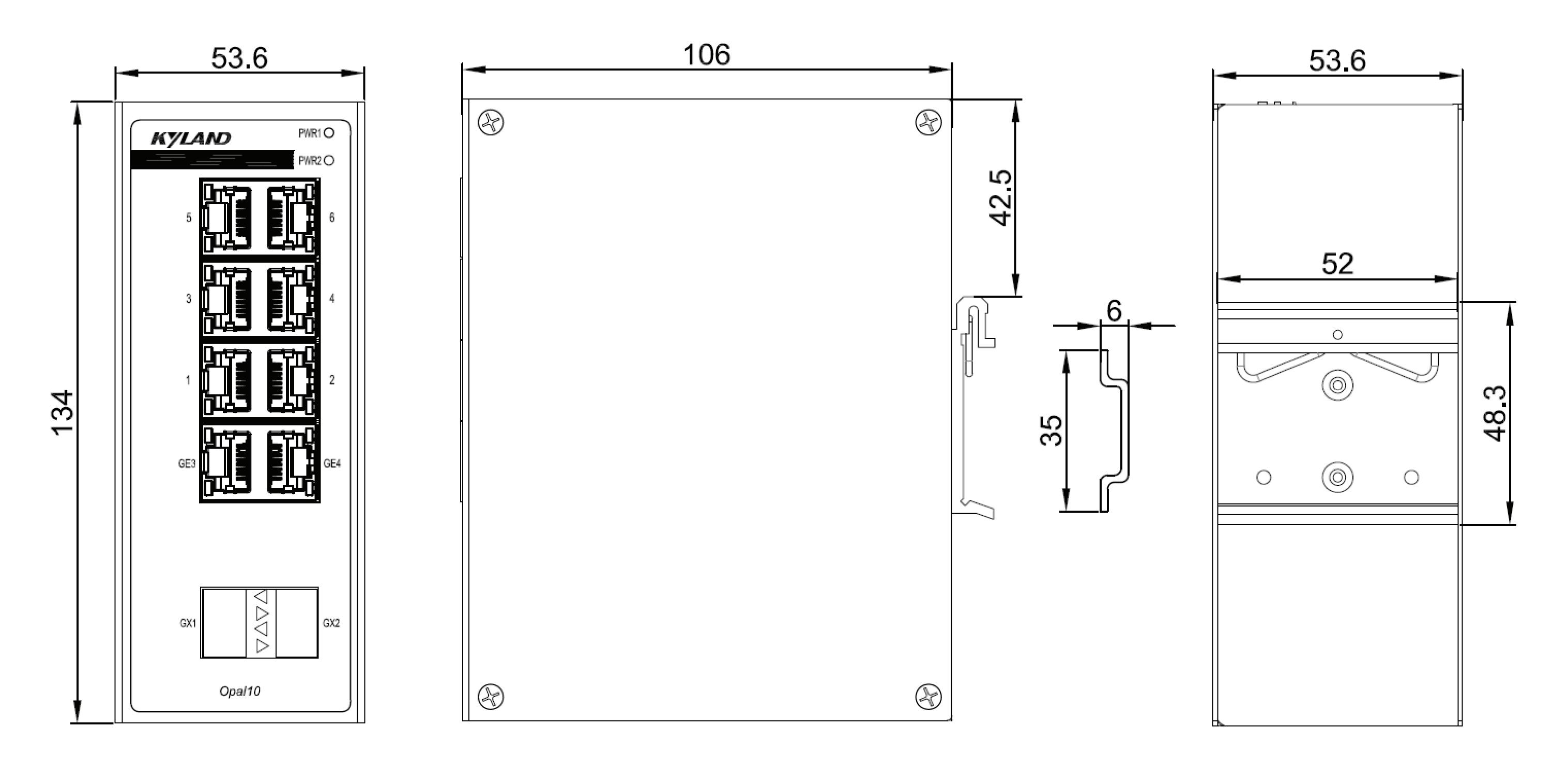
Figure 3 Opal10 Dimensions for DIN-Rail Mounting (unit: mm)
