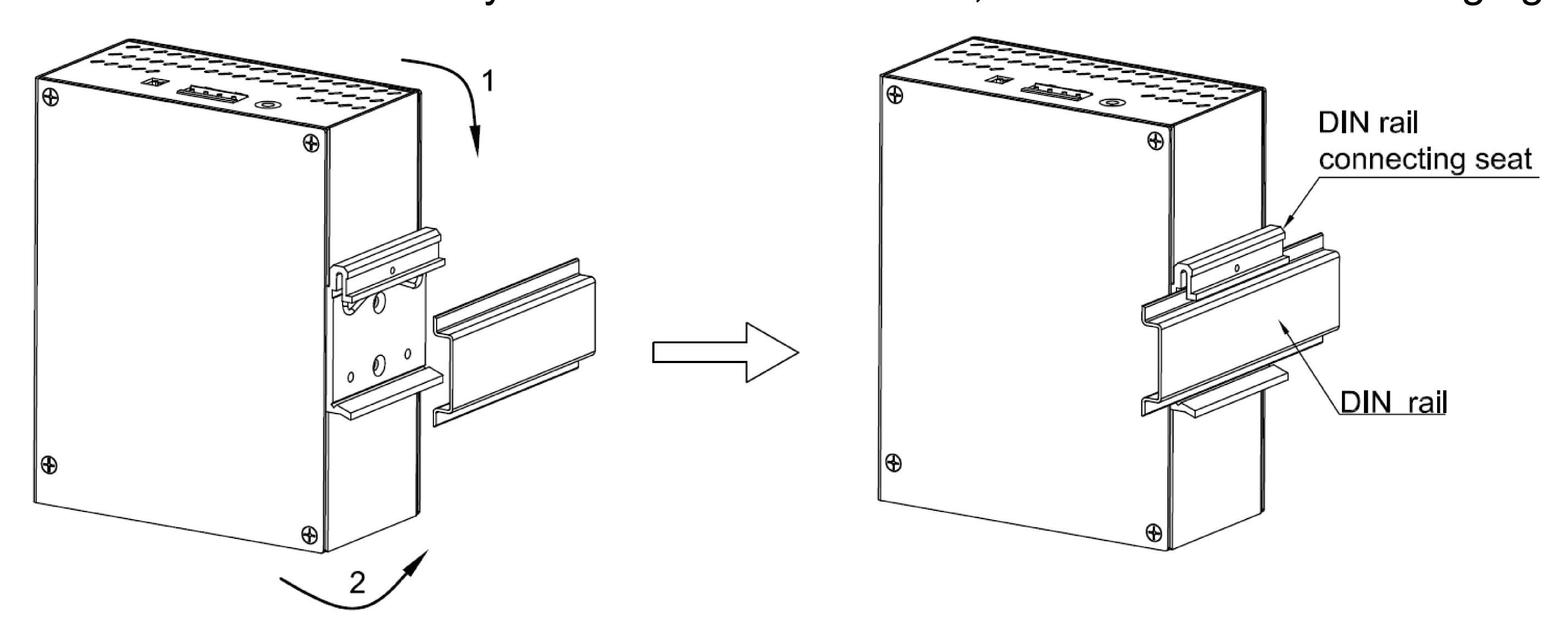
Figure 5 DIN-Rail Mounting
