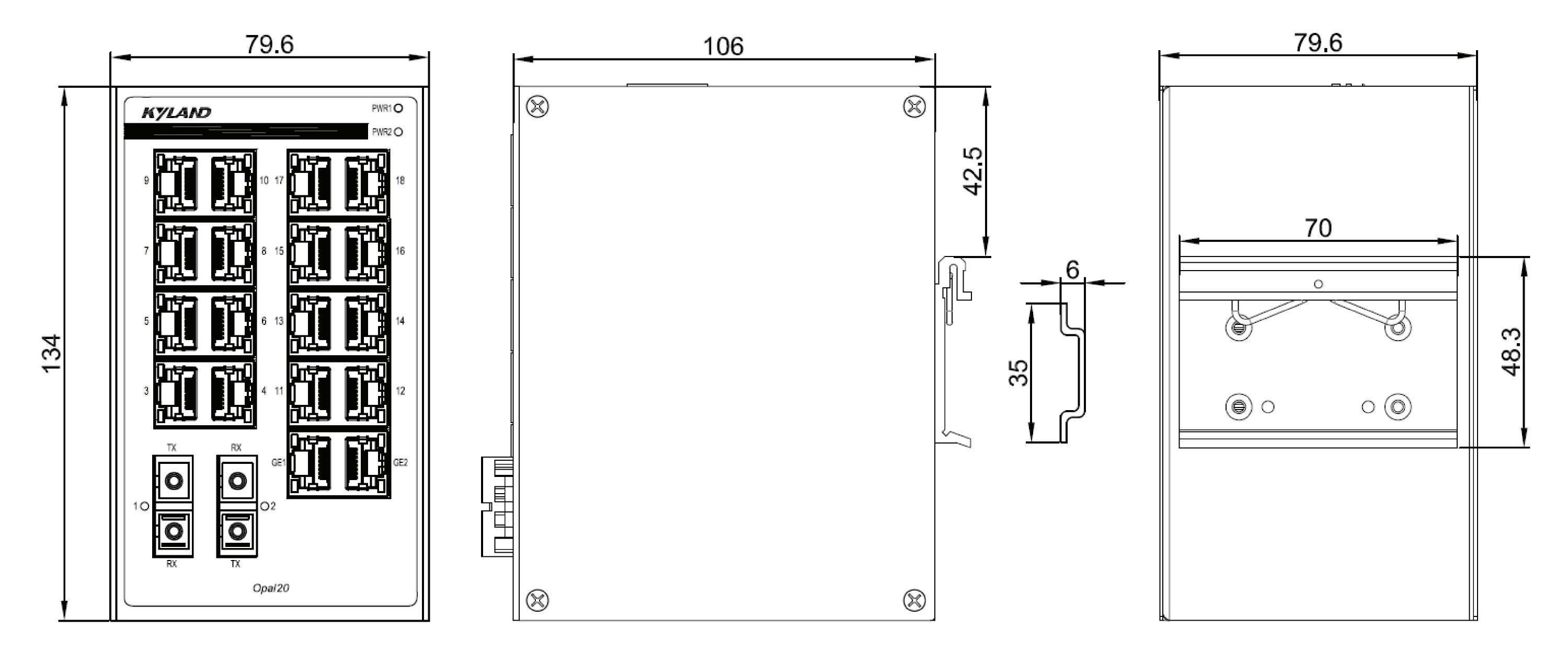
Figure 4 Opal20 Dimensions for DIN-Rail Mounting (unit: mm)
