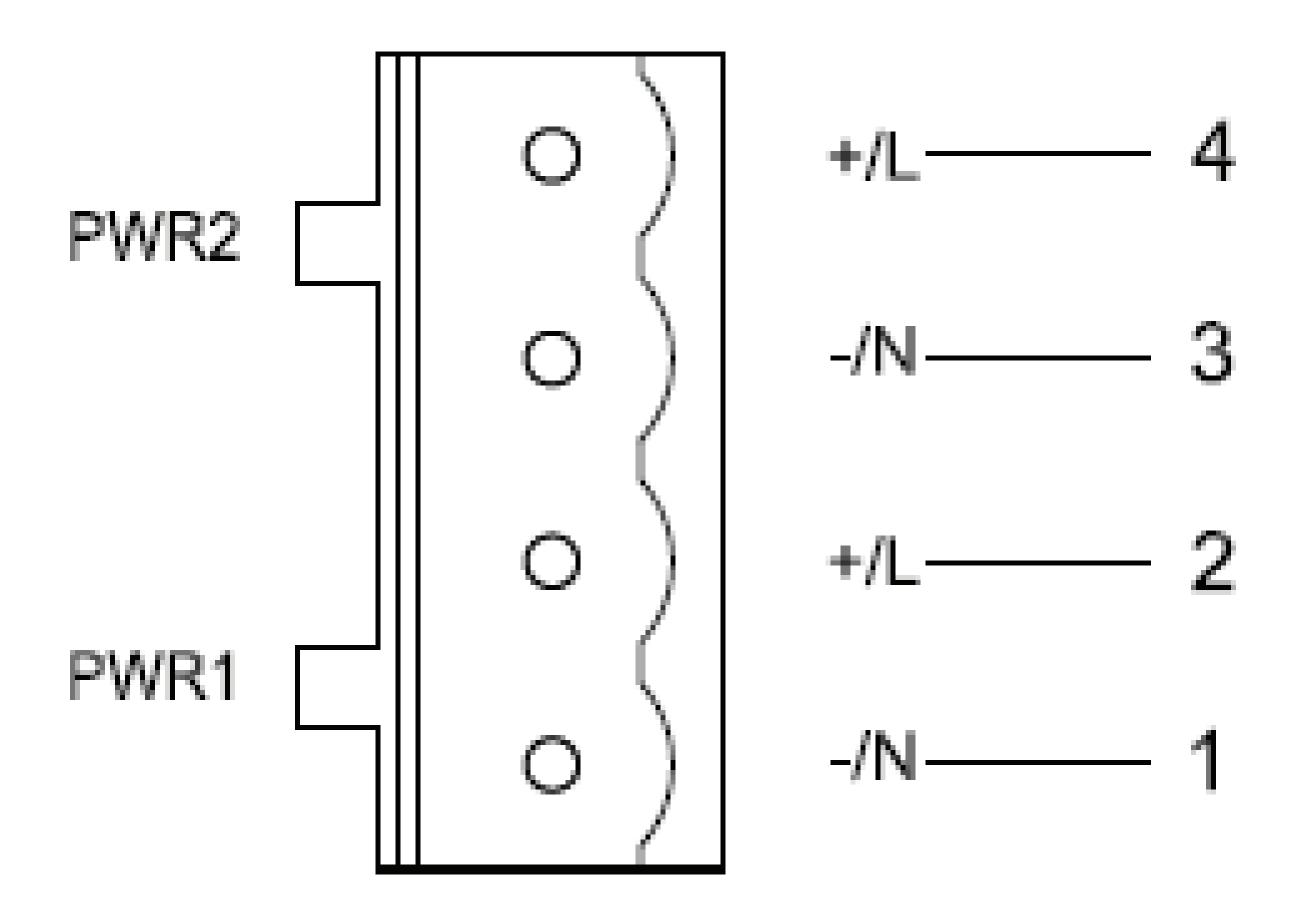
Figure 15 4-Pin 5.08mm-Spacing Plug-in Terminal Block (socket)
