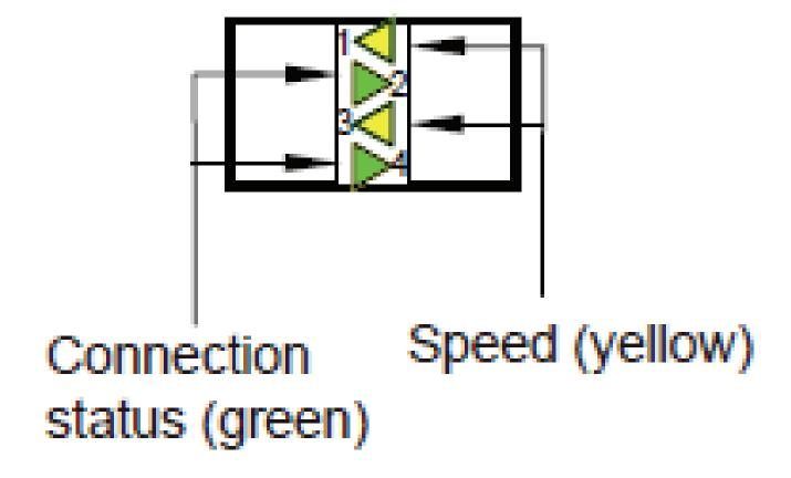
LED 1 and LED 2 indicate the status of the left SFP slot, while LED 3 and LED 4 indicate the status of the right SFP slot.
