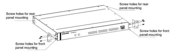
Figure 5 Installing Mounting Brackets
