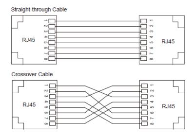
Figure 8 Connection Using Straight-through/Cross-over Cable
