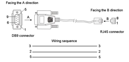
Figure 15 Wiring Sequence of DB9-RJ45 Console Cable
