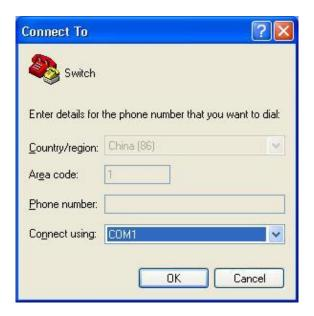
Figure 19 Selecting the Communication Port in Use
