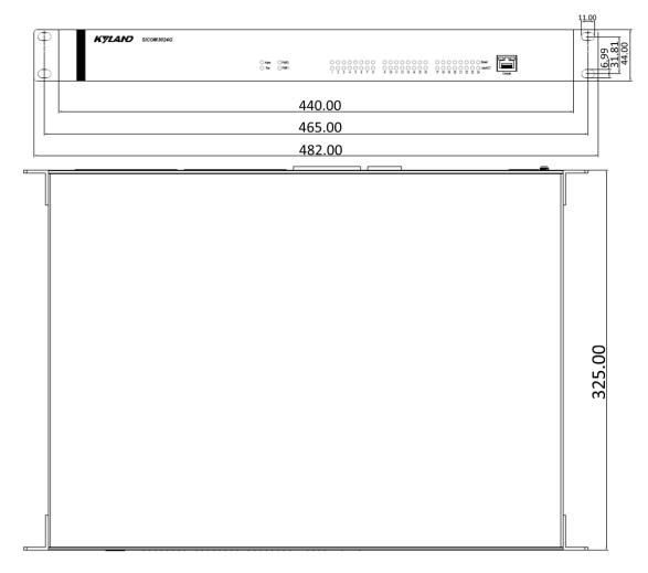
Figure 3 Dimension Drawing (unit: mm)
