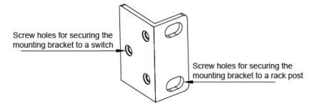
Figure 4 Mounting Bracket
