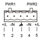
Figure 16 5-Pin 5.08mm-Spacing Plug-in Terminal Block
