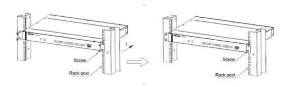
Figure 6 Mounting by Front Panel
