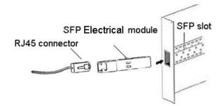
Figure 13 Connecting the Gigabit SFP Electrical Module
