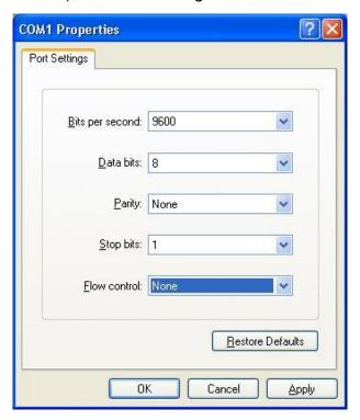
Figure 20 Setting Port Parameters
