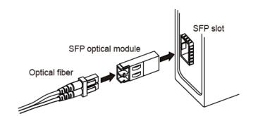
Figure 11 Connecting the Gigabit SFP Optical Module
