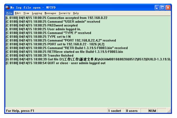
Figure 17 Normal Communication between FTP Server and Switch
