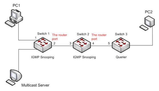
Figure 295 IGMP Snooping Application Example
