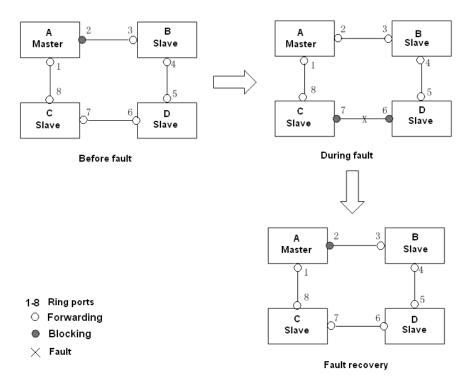
Figure 142 CD Link Fault
