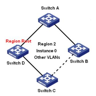
Figure 183 Other VLAN Mapping to Instance 0
