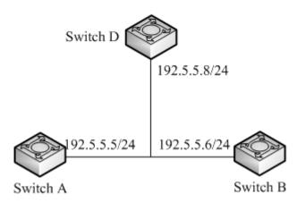
Figure 360 Networking in Multicast Mode
