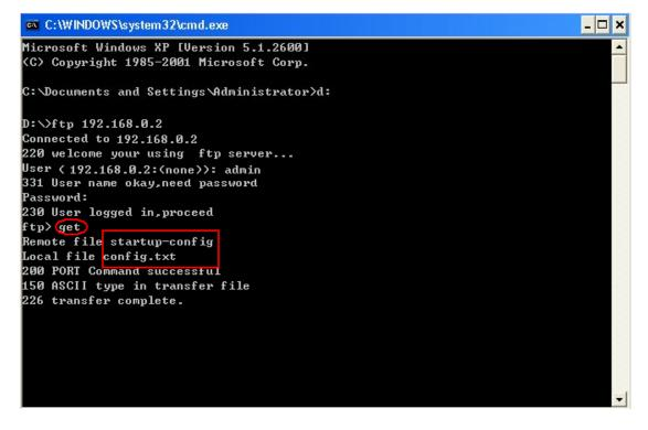
Figure 96 Downloading File from Switch to Client
