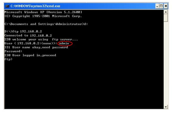
Figure 95 Logging in to the FTP Server
