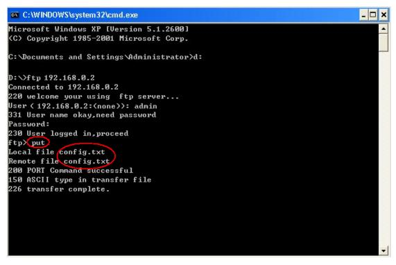
Figure 97 Uploading File from Client to Switch
