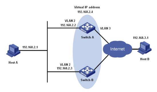
Figure 345 VRRP Typical Configuration Example
