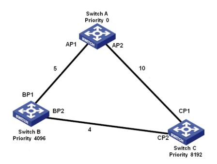
Figure 157 RSTP Configuration Example
