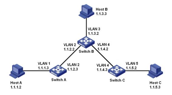
Figure 211 Example for Configuring Static Routes
