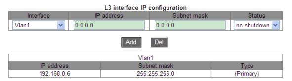
Figure 260 DHCP Client Obtain IP Address-1
