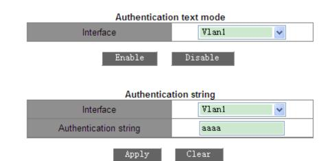
Figure 343 Setting VRRP Authentication Parameters
