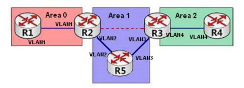
Figure 244 OSPF Typical Configuration Example
