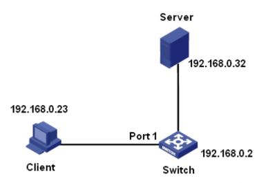
Figure 378 IEEE802.1x Configuration Example
