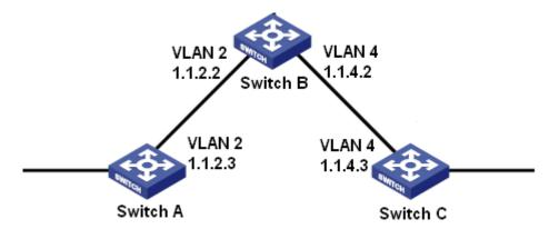
Figure 219 RIP Configuration Example
