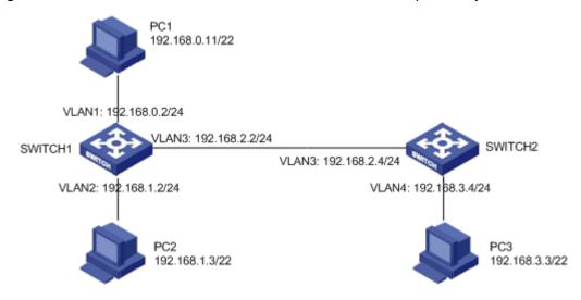
Figure 122 Proxy ARP Configuration Example
