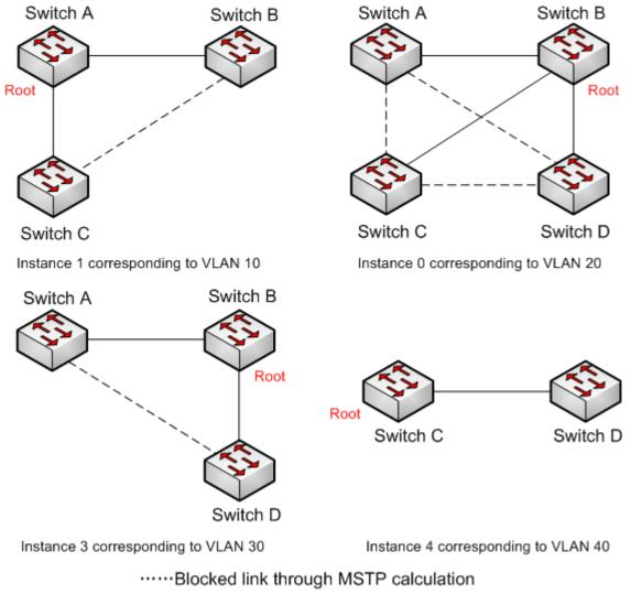
Figure 195 Spanning Tree Instance of each VLAN
