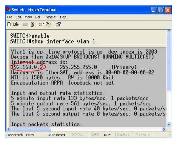
Figure 123 Displaying IP Address
