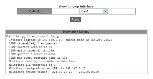
Figure 307 the Information of IP IGMP Interface
