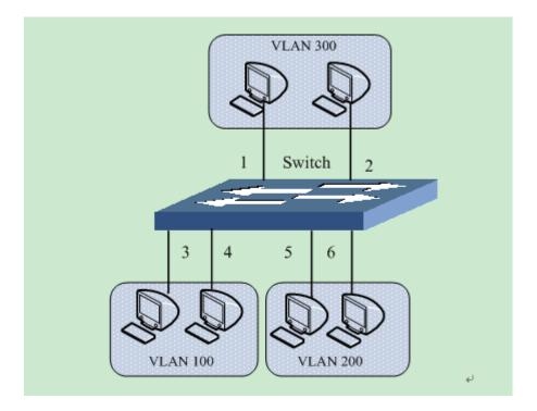
Figure 50 PVLAN Configuration Example
