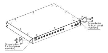
Figure 4 Installing Mounting Brackets
