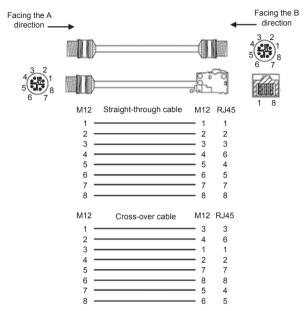
Figure 11 Connection Using Straight-through/Cross-over Cable
