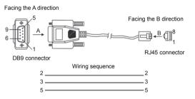
Figure13 Wiring Sequence DB9-RJ45 Console Cable
