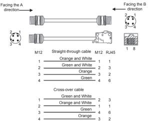
Figure 8 Connection Using Straight-through/Cross-over Cable
