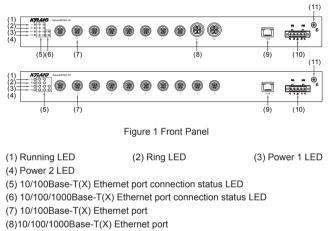
(9) Console port (10) Power terminal block (11) Grounding screw
