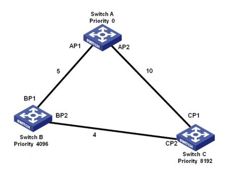
Figure 211 RSTP Configuration Example
