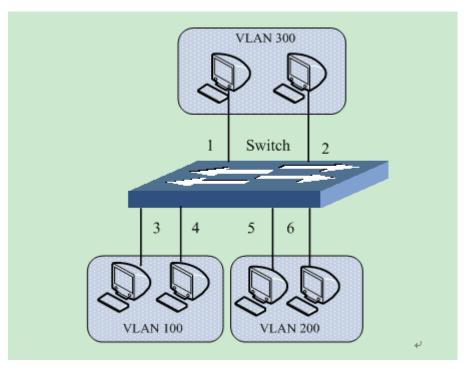
Figure 183 PVLAN Configuration Example
