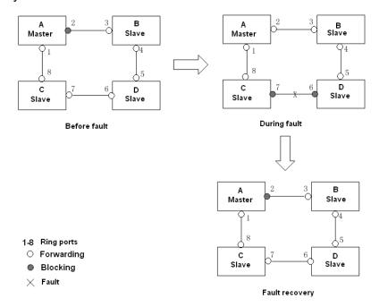
Figure 189 CD Link Fault
