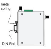
To remove the AWK-1131A from the DIN-Rail, simply reverse Steps 1 and 2.
