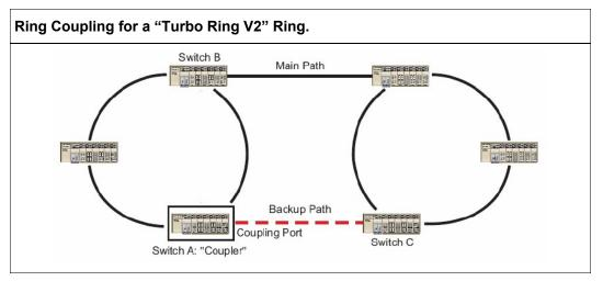
Note that the ring coupling settings for a "Turbo Ring V2" ring are different from a "Turbo Ring" ring. For Turbo Ring V2, Ring Coupling is enabled by configuring the "Coupling Port (Primary)" on Switch B, and the "Coupling Port (Backup)" on Switch A only. You do not need to set up a coupling control port, so that a "Turbo Ring V2" ring does not use a coupling control line.
