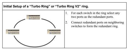
The user does not need to configure any of the switches as the master to use Turbo Ring or Turbo Ring V2. If none of the switches in the ring is configured as the master, then the protocol will automatically assign master status to one of the switches. In fact, the master is only used to identify which segment in the redundant ring acts as the backup path. In the following subsections, we explain how the redundant path is selected for rings configured for Turbo Ring, and Turbo Ring V2.
