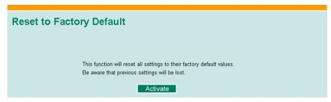
The Factory Default function is included to give users a quick way of restoring the EDS-728's configuration settings to their factory default values. This function is available in the Console utility (serial or Telnet) and Web Browser interface.
