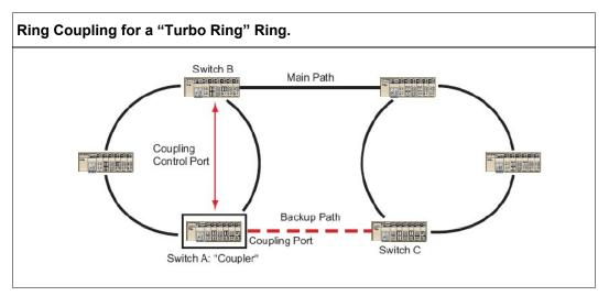
To configure the Ring Coupling function for a "Turbo Ring" ring, select two EDS-728 units (e.g., Switch A and B in the above figure) in the ring, and another two EDS-728 units in the adjacent ring (e.g., Switch C and D).
