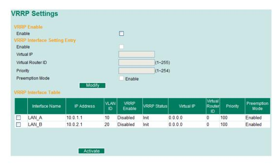
The Virtual Router Redundancy Protocol (VRRP) feature can solve the static configuration problem. VRRP enables a group of routers to form a single virtual router with a virtual IP address. The LAN clients can then be configured with the virtual router's virtual IP address as their default gateway. The virtual router is the combination of a group of routers, and also known as a VRRP group.
