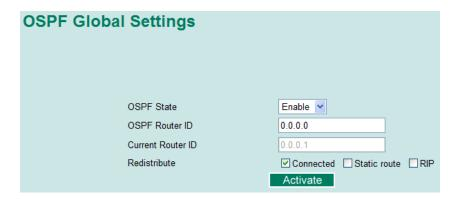
Each L3 switch/router has an OSPF router ID, customarily written in the dotted decimal format (e.g., 1.2.3.4) of an IP address. This ID must be established in every OSPF instance. If not explicitly configured, the default ID (0.0.0.0) will be regarded as the router ID. Since the router ID is an IP address, it does not have to be a part of any routable subnet in the network.
