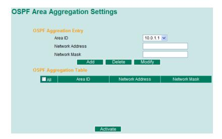
Each of OSPF areas which consist of a set of interconnected subnets and traffic across areas is handled by routers attached to two or more areas, known as Area Border Routers (ABRs). With OSPF aggregation function, users can combine groups of routes with common addresses into a single routing table entry. The function is used to reduce the size of routing tables.
