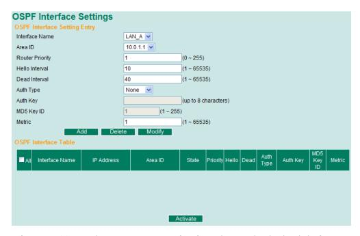
Before using OSPF, we have to assign an interface for each area. Also the detailed information of the interface can be defined in this section. See the details in the following descriptions:
