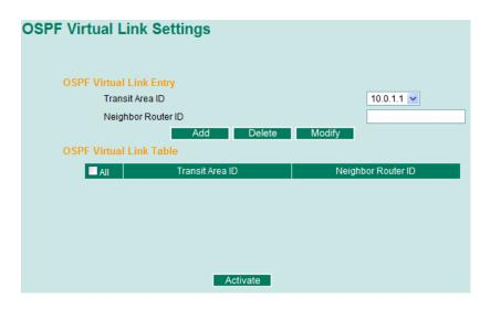
All areas in an OSPF autonomous system must be physically connected to the backbone area (Area 0.0.0.0). However, this is impossible in some cases. For those cases, users can create a virtual link to connect to the backbone through a non-backbone area and also use virtual links to connect two parts of a partitioned backbone through a non-backbone area.
