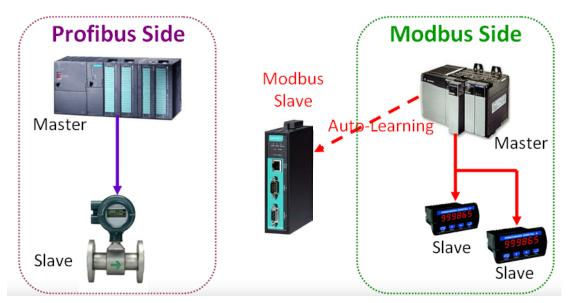
After some time, MGate 4101-MB-PBS will fully learn the requests from the Modbus master. Through this QuickLink process, the MGate 4101-MB-PBS can replace the legacy Modbus master. Moreover, the MGate 4101-MB-PBS can respond to all of the Modbus slaves correctly.
