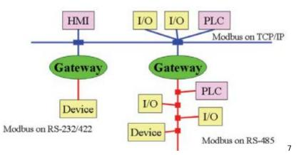
Ordinarily, Modbus TCP and Modbus ASCII/RTU are unable to communicate with each other.
