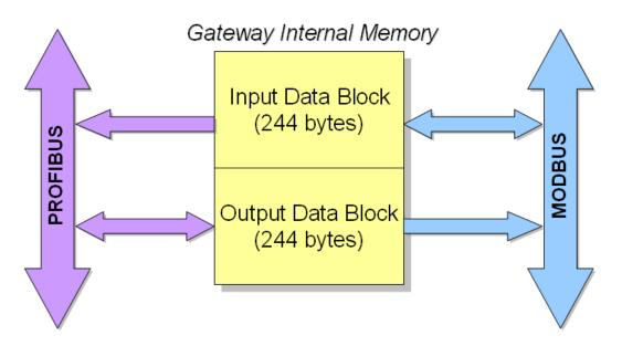
Before data exchange, you first need to map Modbus requests to the I/O module. In troubleshooting, understanding the relationships between the I/O modules and memory is a good way to exclude wrong IO configuration issues. The IO Map function provides a way to check the internal memory address. You can open the IO map dialog with the **IO Map** button.
