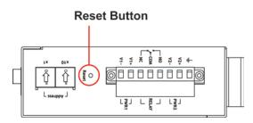
To reset the MGate to the factory default settings, hold down the reset button for about 5 seconds. The MGate will restart and be rest to factory default settings.
