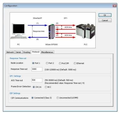
You can configure the options for DF1, EtherNet/IP, and CIP protocol. Response Time-out defines how much time the EIP3000 needs to wait for a response after sending a PCCC command to a DF1/EIP device. We strongly suggest that the value should be greater than ACK timeout, since it requires at least double the timeout values of DF1 ACK after the EIP3000 forwards a PCCC command and before it gets a response.
